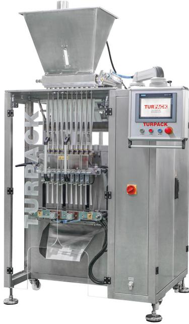
This machine is designed to fill free flowing products such as sugar, salt, spices and black pepper through volumetric cups into affixed three side sealed stickpack. The volume of the product feed into the volumetric containers can be adjusted between a certain weight ranges, this assures that the desired weight is sensitively filled into the stickpack.
